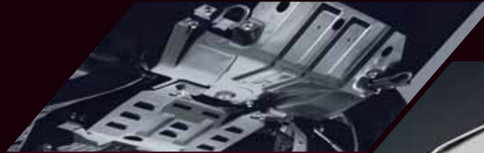
Underbody Steel Skid Plate
