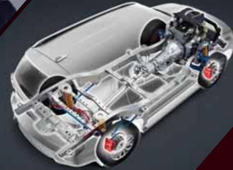
Heavy - duty Ladder Construction Chassis
